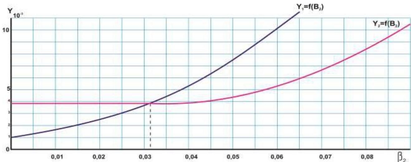
Fig 3. Determination of the value of  $\beta_2$  by the transcendental equation.
